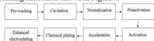
Figure 4. The chemical plating process on the surface of the insulating material
